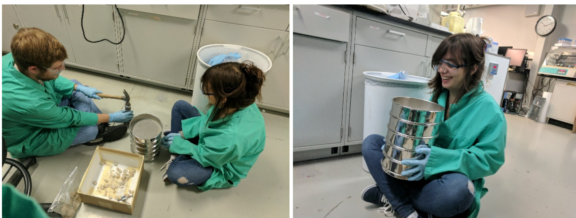
Figure 4. Images of Frances Zengotita and another LANL intern crushing and sieving dolomite rocks.
