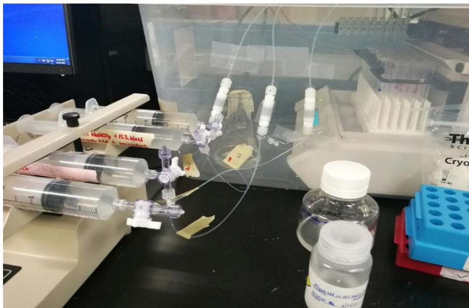
Figure 7. Experimental setup with syringe pump (0.013 mL/min) and fraction collector.
