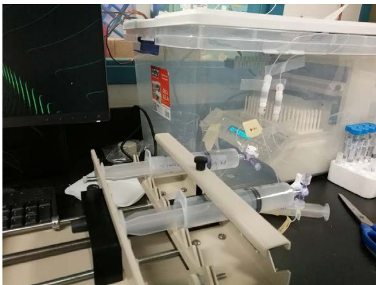
Figure 8. Image of the experimental setup for Cs experiments with two syringes (one for stressed and one for viable bacteria) connected to syringe pump and injected into columns with effluent collection in the fraction collector in a makeshift humidity chamber.
